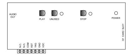
Power Input: VDC & GND
