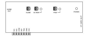
6. Press the PGM button again to exit the programming mode. Both the audio and the relay will be forced off upon exit. The PGM light will also be turned off to indicate that the unit is no longer in the programming mode. The unit will exit the programming mode automatically if the maximum cycle time is exceeded.
