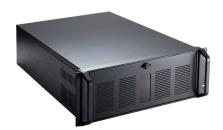
eALog is an open platform voice logger built with cutting edge technologies. It is capable of passively tapping into digital or analog phone lines for real-time call recording and/or monitoring without any noticeable interruption in the service. Recordings are stored internally and can be retrieved locally or remotely via telephone or LAN. eALog can be purchased as a turnkey system complete with application software, or with SDK (software development kit) for building your own system.
