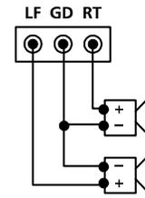
The left channel signal is internally inverted and that's why the left speaker has an inverted polarity for regular stereo output. If the left speaker is not inverted then the output is virtual surround stereo.
