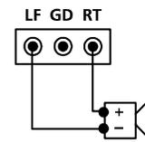
Since BTL mono provides four times the output power of regular mono at the same supply voltage, it is often used to boost the output power when the supply voltage is low. However, the speaker impedance should not be lower than 8 Ohms to avoid overloading the power amp.
