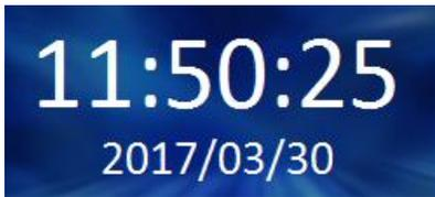
A white clock indicates that the PC has linked with the NTP-100 and the GPS is working properly.
