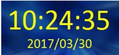
A yellow clock indicates that the PC has linked with the NTP-100 but the GPS is not working properly.
