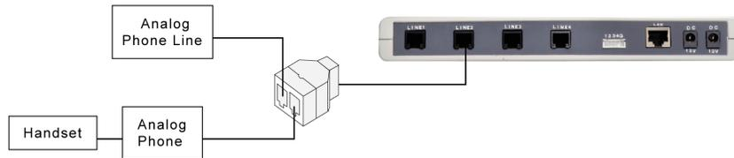
Use the supplied Y connectors and connect up to four lines to the logger via the jacks labeled LINE 1 ~ LINE 4. Analog lines can be connected to the logger directly. Digital lines cannot be recorded.
