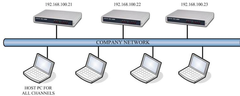
When a single host computer is used all record data is stored on it, allowing for centralized system management. In this scheme the host computer is usually dedicated for the sake of better performance since there may be many channels to serve. Although the diagram above shows a shared network, it is recommended to put the dedicated host computer on a dedicated network with the loggers for maximum performance and security.
