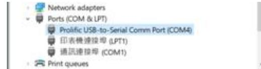
To correct the COM Port setting error, close the software first then open *FMScancfg.ini* with a text editor and correct the [COM] number. Save the file and run the software again.
